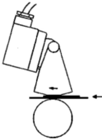
A double sheet strikes the scanner on the microswitch, interrupting the sheet flow-through.
