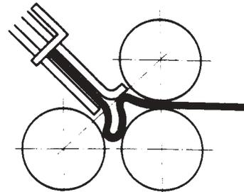
Thin weak papers require a small buckle space and a narrow buckle-plate.
