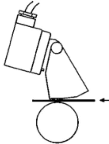
With single sheet thickness, the scanner remains untouched and sheets move freely.
