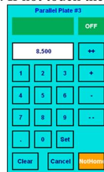
Use the keypad or the + or – buttons to correct the fold. You can enter a new value and touch set or touch the +, ++, - or – to adjust the fold. Run three more sheets and repeat this step until the paper is folded exactly in half.
