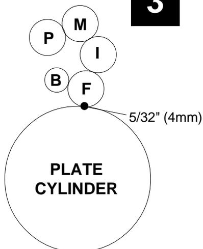
Drop the water form roller to the plate and check the stripe. It should be  $\frac{5}{32}$ " (4mm). Adjust the stripe using the stop screws on the dampener frame (subject arrow). **Turning the screw down decreases the stripe.** Lock in place using lock nut.
